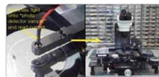
"Photo detector" test system with probe station
