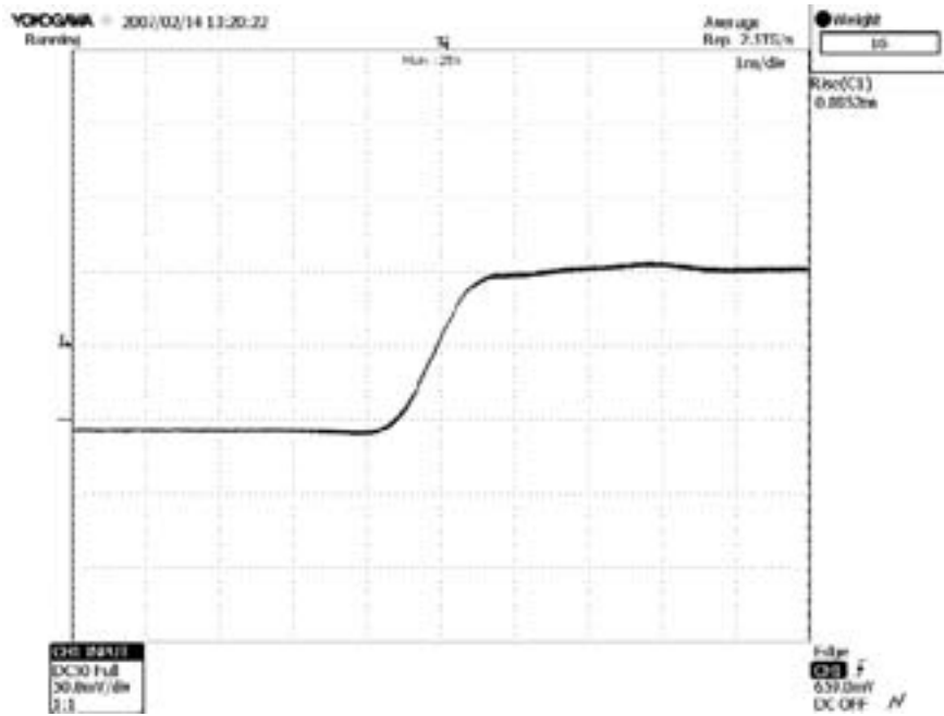
Large Signal Response output signal for 100 MHz, 200 μW modulated optical input signal (with 4 times averaging)
