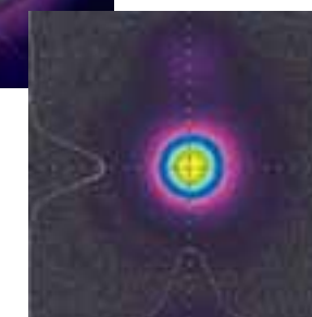
Near field beam profile of TEM 00 at 1064nm.
